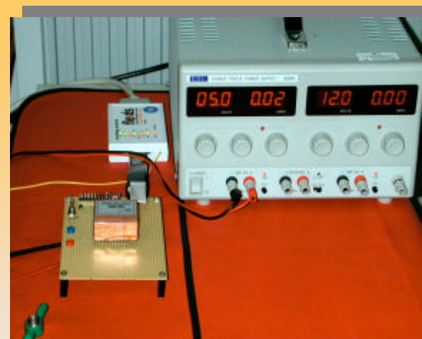
(LEFT) uDPU during memory test (500 mW on primary). (RIGHT) uDPU in stand-by (100mW on primary).
