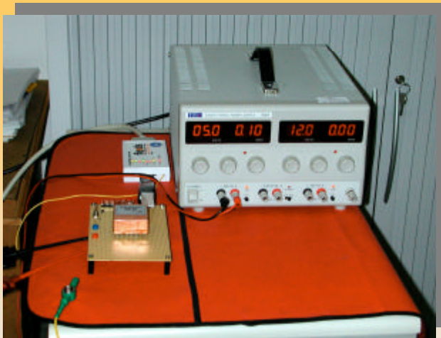
(LEFT) uDPU during memory test (500 mW on primary). (RIGHT) uDPU in stand-by (100mW on primary).
