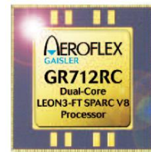
Dual-Core LEON 3FT SPARK V8 32-bit
